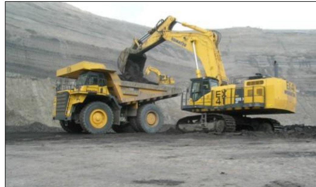
One (1) Komatsu PC1250 excavators 7 cu.m. bucket capacity
