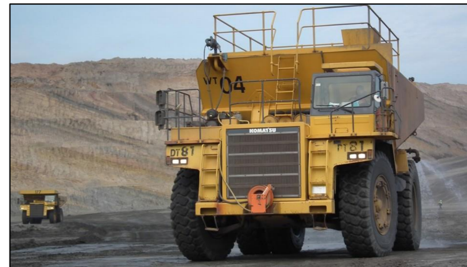
Five (5) Units Komatsu water trucks (4) Units - 70,000 liters capacity (1) Units 40,000 liters capacity
