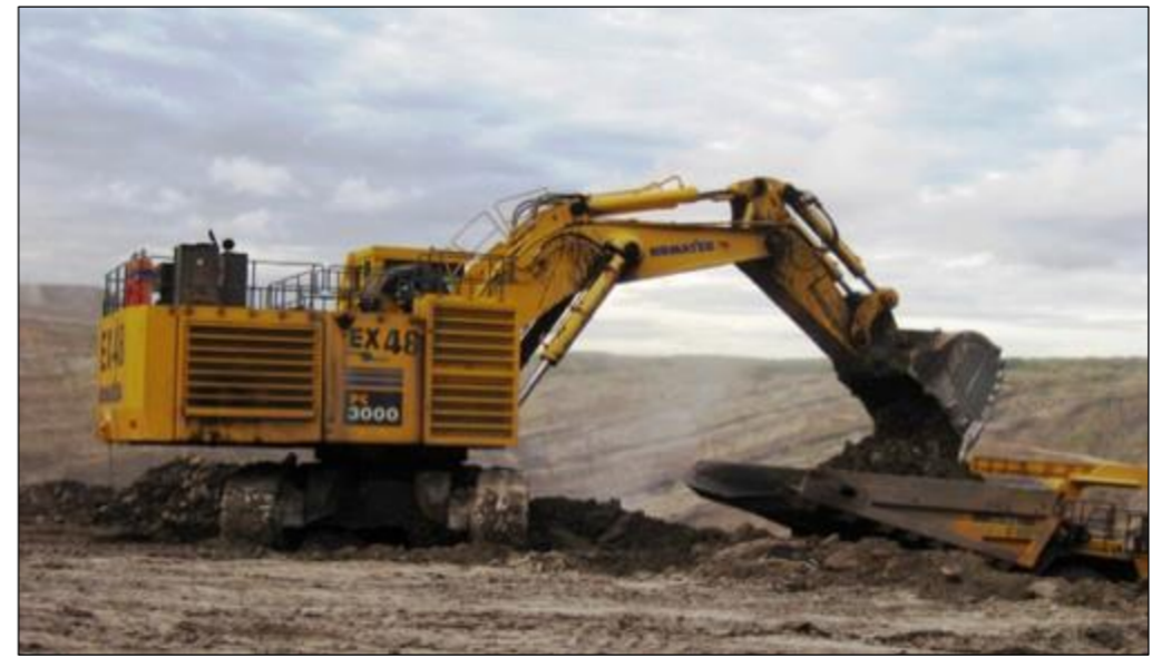
Eighth (8) units Komatsu PC3000 Excavator 15 cu.m. bucket capacity
