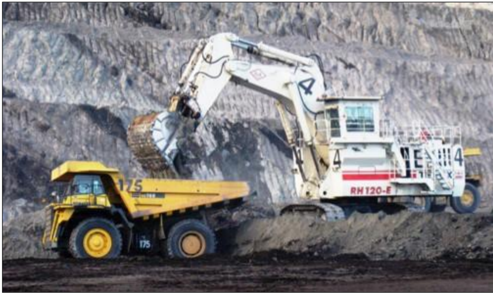
Four (4) Excavator 0 & K RH-120 16 cu.m. bucket capacity
