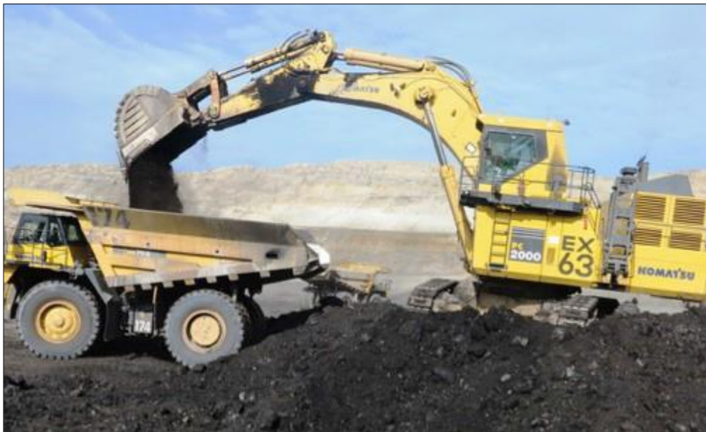
Eighth (8) Komatsu PC2000 excavators 12 cu.m. bucket capacity
